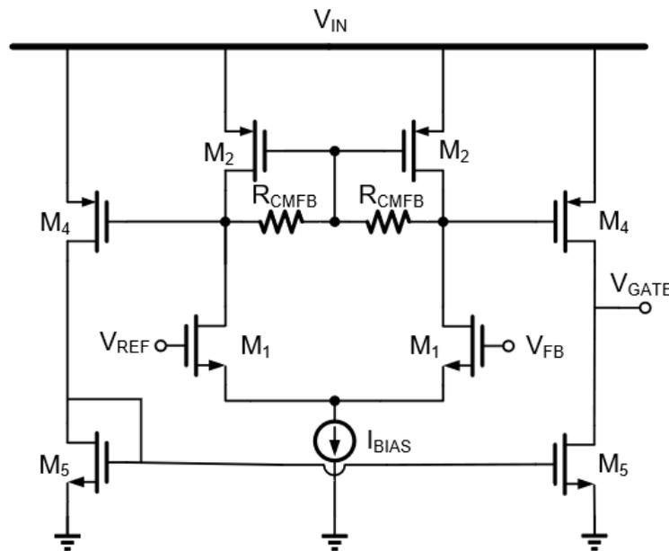
Figure 3.8: Two-stage error amplifier schematic
