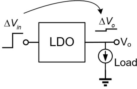
Figure 2.3: Line regulation diagram
