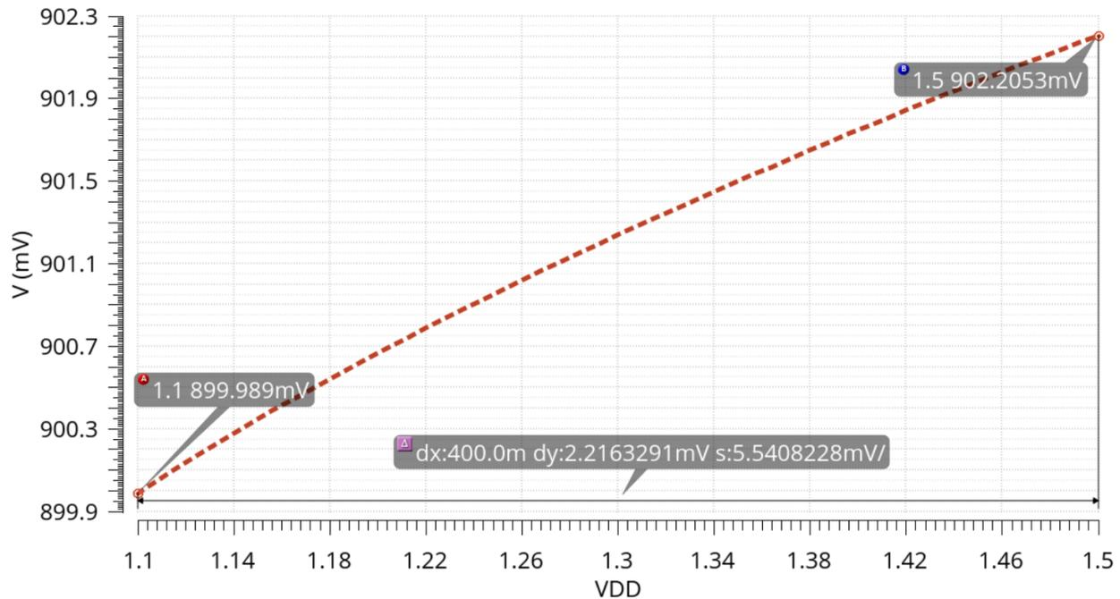
Figure 4.3: Line regulation at 0 A load current
