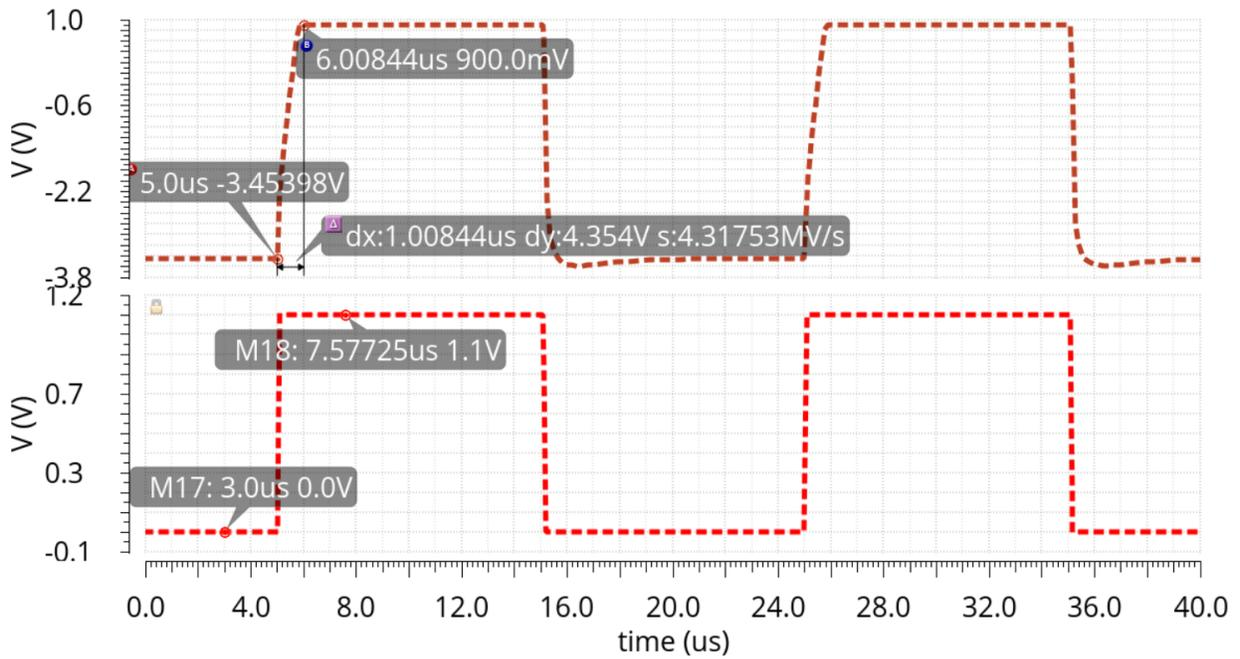
Figure 4.10: Startup condition with 100 mA load current
