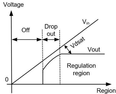
Figure 2.2: Input-output voltage characteristics of a typical LDO
