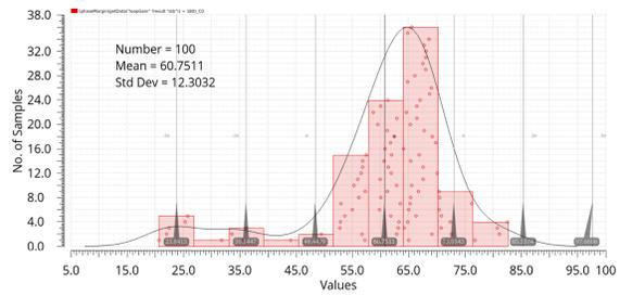
Figure 4.14: Phase margin for 1 mA load
