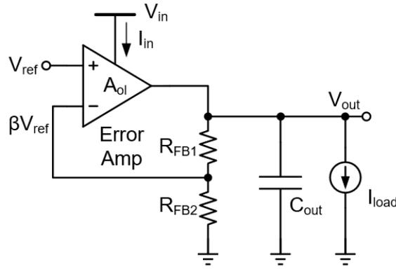
Figure 2.1: Block diagram of a typical LDO
