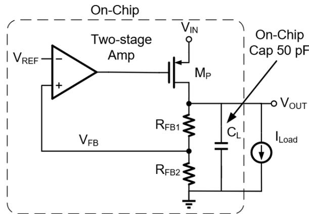
Figure 3.2: Macro model of the uncompensated LDO
