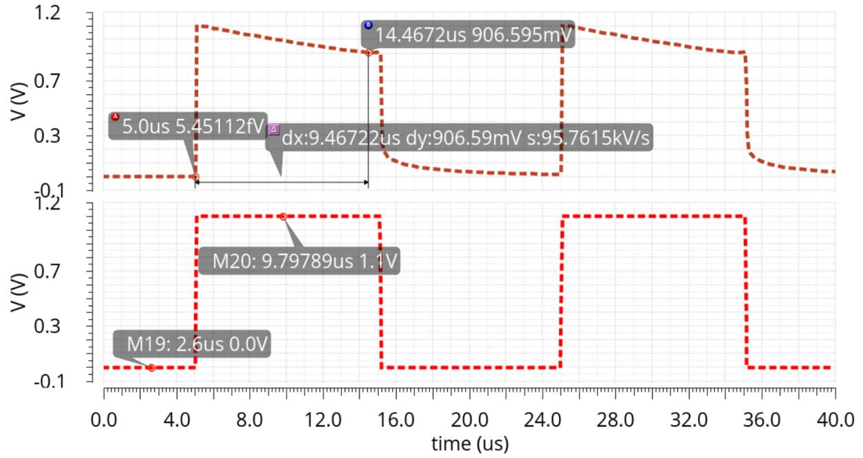
Figure 4.9: Startup condition with 0 A load current
