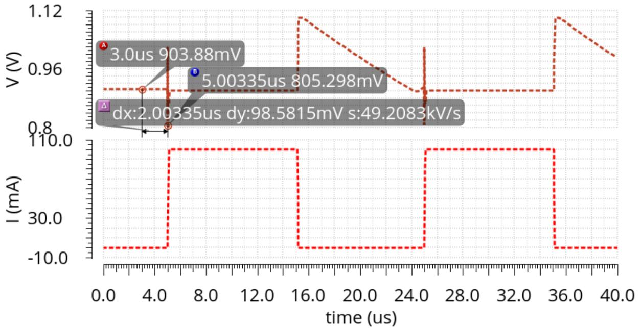
Figure 4.6: Compensated load transient response
