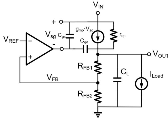
Figure 3.20: PMOS LDO pass element small signal model
