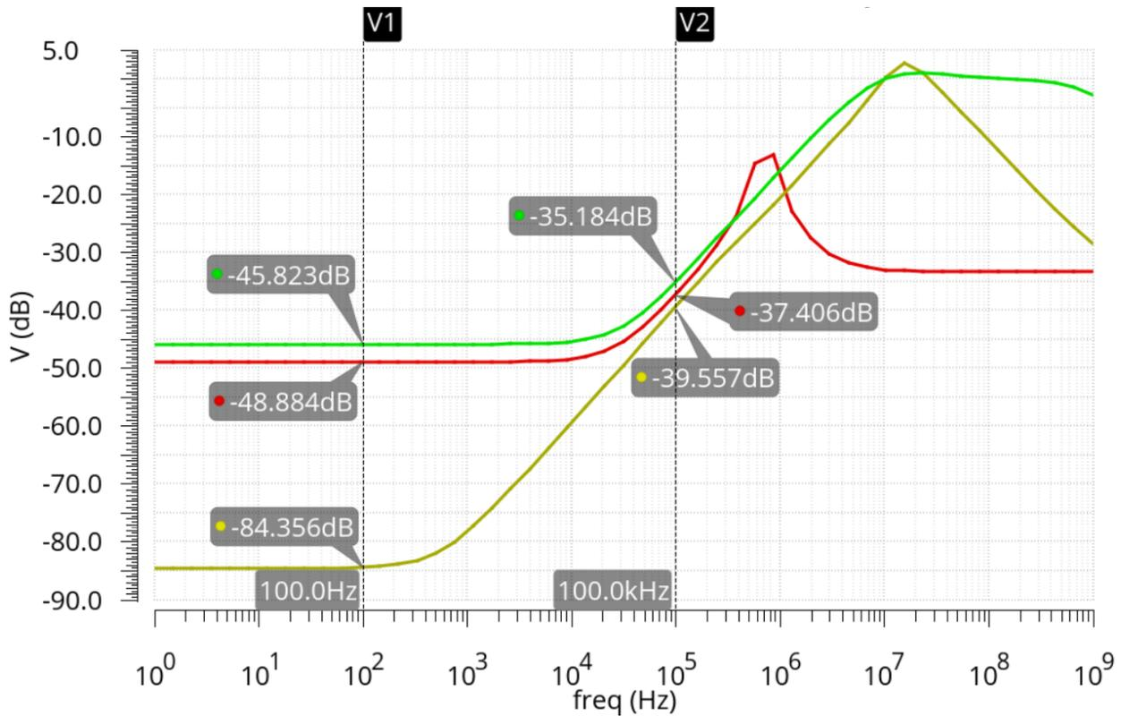
Figure 4.4: PSRR at 0, 1 mA and 100 mA load current
