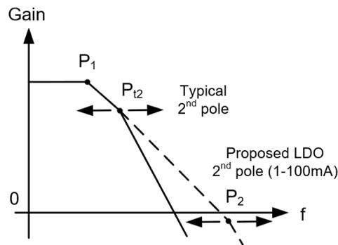
Figure 3.24: Capacitor-less LDO output pole movement
