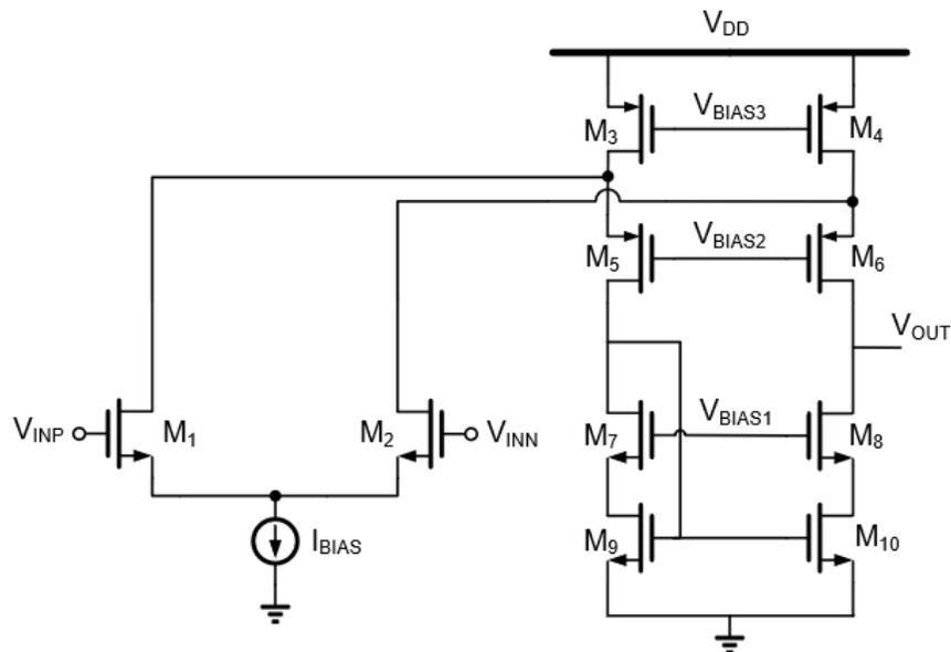
Figure 3.7: Low voltage folded-cascode OTA
