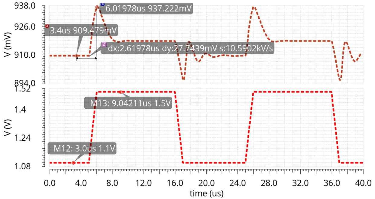
Figure 4.7: Line transient response at no load
