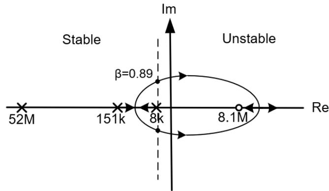
Figure 3.28: Root locus for sweeping feedback factor at no load
