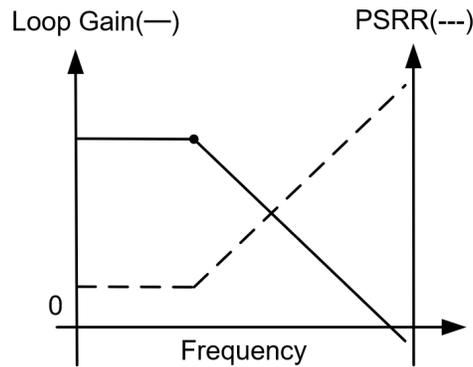
Figure 2.5: PSRR with frequency
