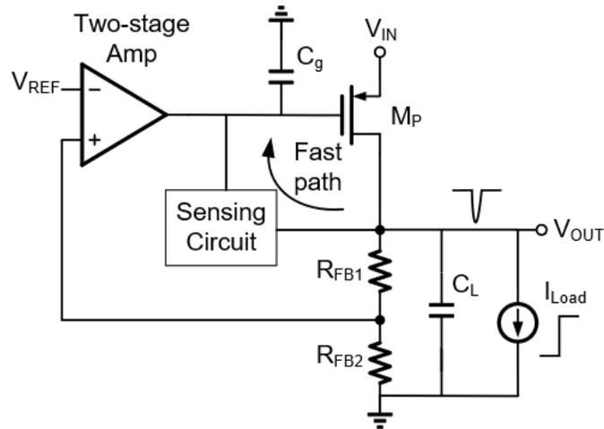
Figure 3.14: Transient-enhanced circuit concept
