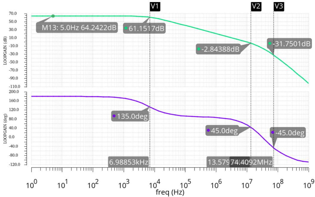
Figure 3.29: Frequency response for sweeping feedback factor at 1 mA load
