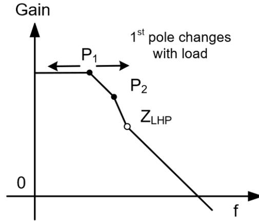
Figure 2.8: Frequency response of the conventional LDO
