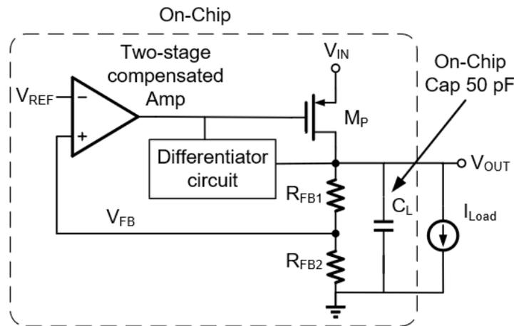
Figure 3.3: Macro model of the compensated LDO
