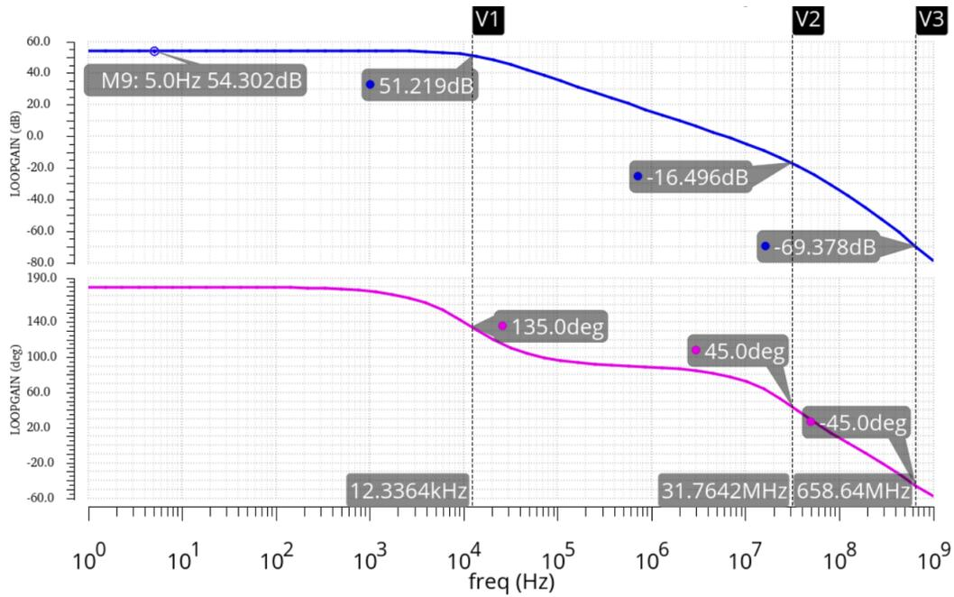
Figure 3.31: Frequency response for 100 mA load
