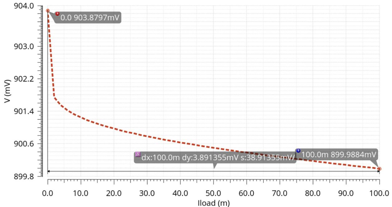
Figure 4.2: Load regulation with load from 0 A to 100 mA
