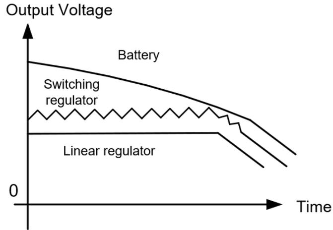
Figure 1.2: Output voltage after battery and different regulator
