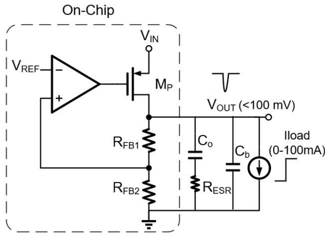
Figure 2.6: Macro model of the uncompensated load transient
