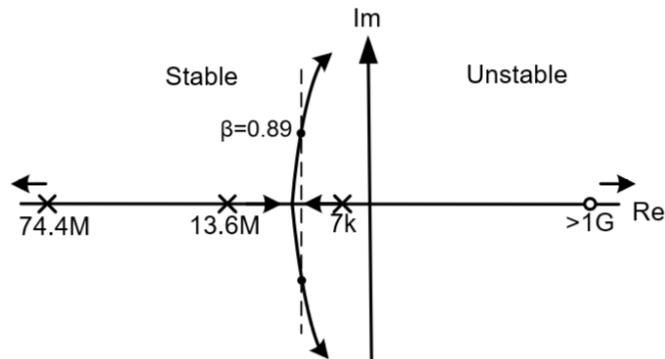
Figure 3.30: Root locus for 1 mA load
