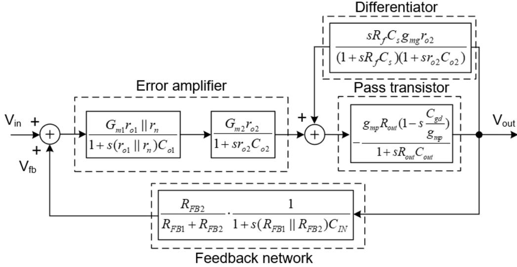
Figure 3.35: Block diagram of the proposed LDO during transients
