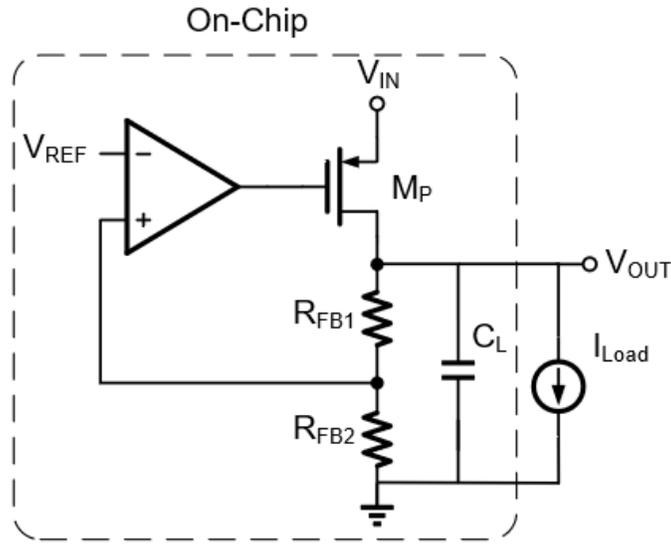
Figure 2.9: External Capacitor-less LDO
