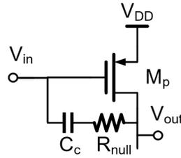
Figure 3.25: Miller compensation with a nulling resistor
