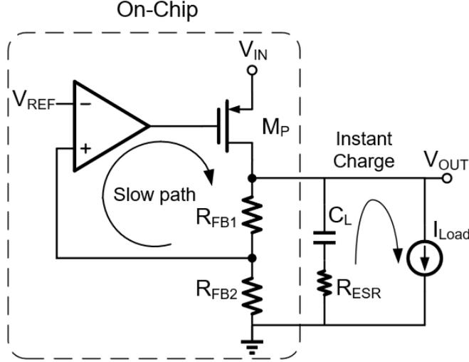
Figure 2.7: Conventional LDO current path during transients
