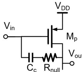
Figure 2.11: Miller compensation with a nulling resistor
