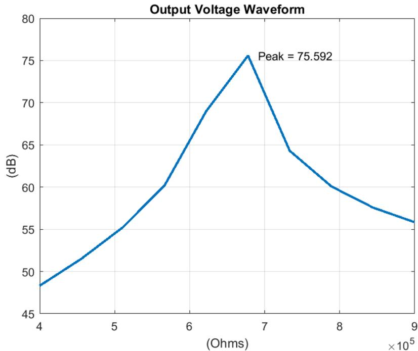
Figure 3.11: Relationship between gain and common mode feedback resistors
