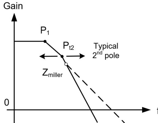
Figure 2.10: A typical AC response of a capacitor-less LDO with an LHP zero
