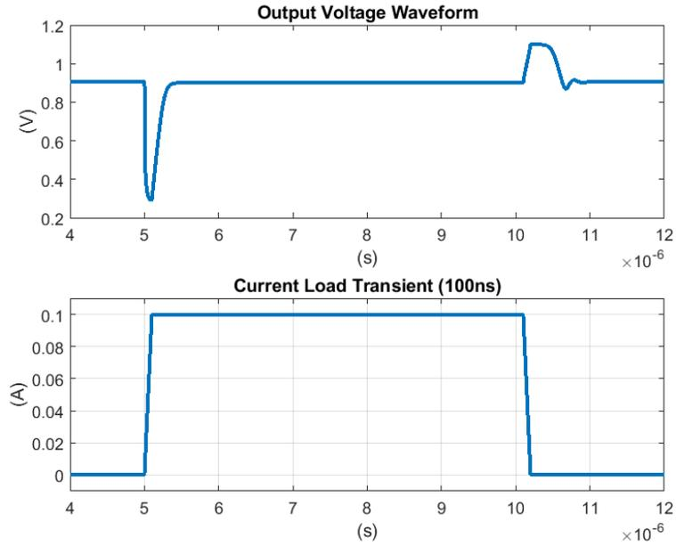
Figure 3.13: Uncompensated transient response
