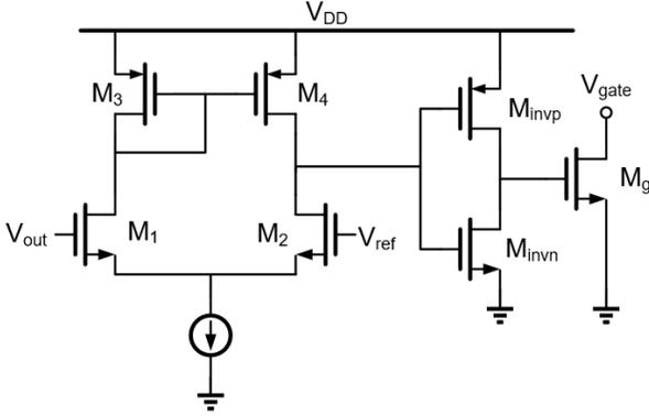
Figure 3.16: Analog comparator
