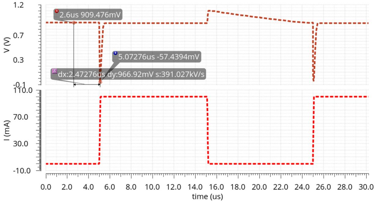
Figure 4.5: Uncompensated load transient response
