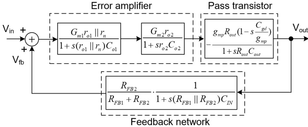
Figure 3.21: Block diagram of the proposed LDO
