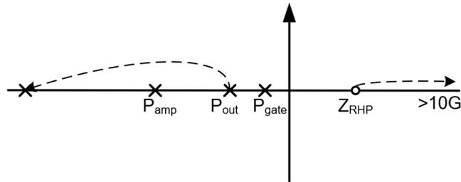
Figure 3.26: Poles and zero movement as load changes from 0 A to 100 mA
