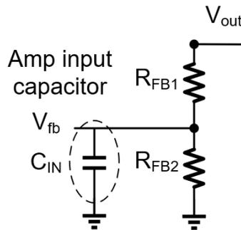
Figure 3.19: Parasitic capacitor in feedback network
