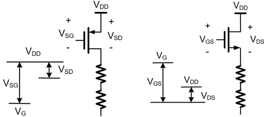
Figure 3.4: Input swing comparison between NMOS and PMOS pass transistors
