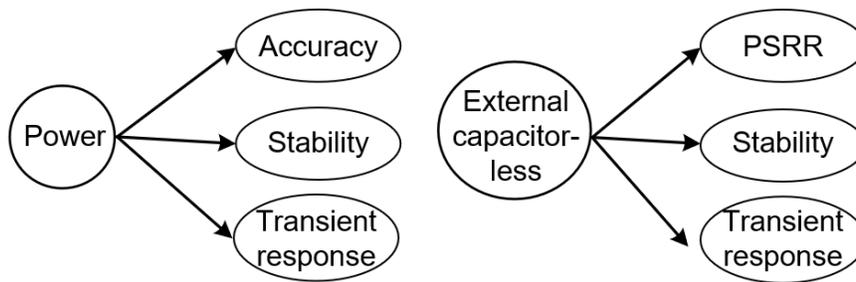
Figure 3.1: Low power external capacitor-less design trade-offs
