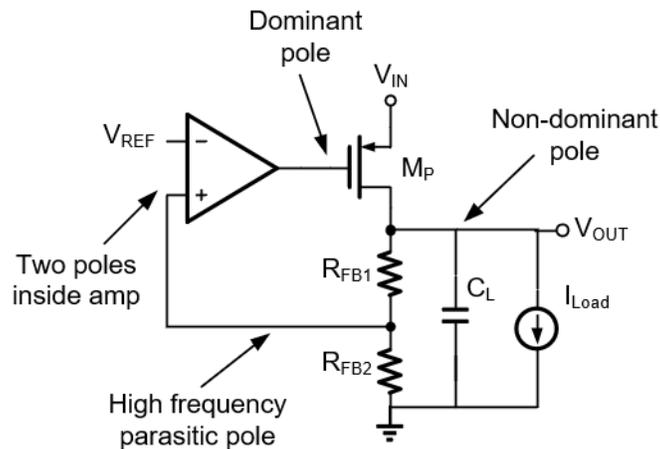
Figure 3.18: Capacitor-less LDO poles location
