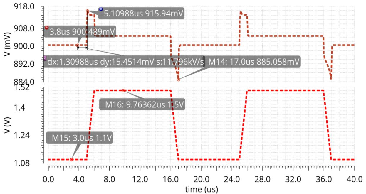
Figure 4.8: Line transient response at 100 mA load
