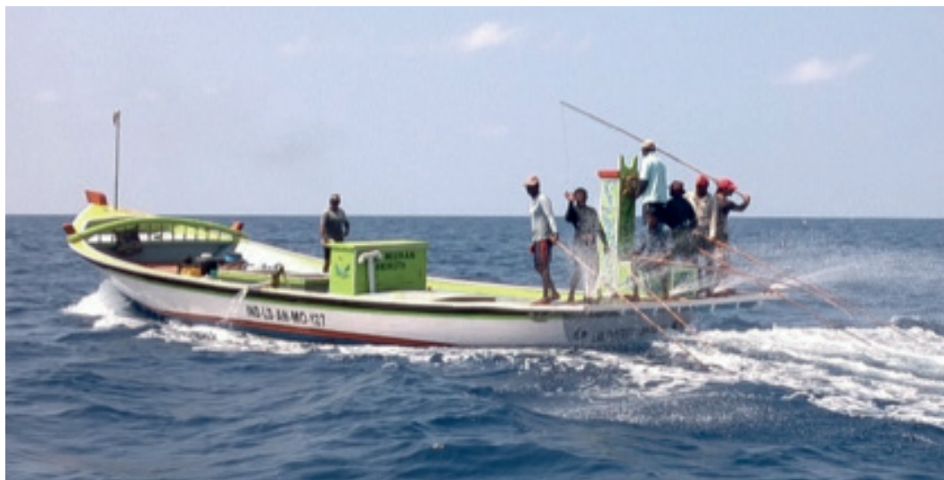
Figure 7. Pole and line boat fitted with mechanical water splasher at stern
