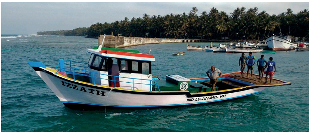
Figure 5. Pole and Line boat modified to Maldivian type boat (initial phase of transformation)
