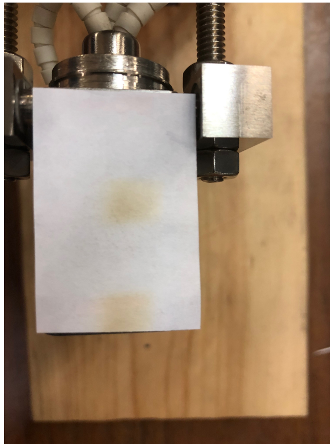
Figure 2.19: Burned paper marking beam spot
