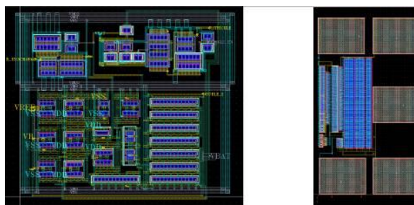
Figure 13. Layout of the battery charger and the DC/DC boost converter in CMOS 0.25um technology.
