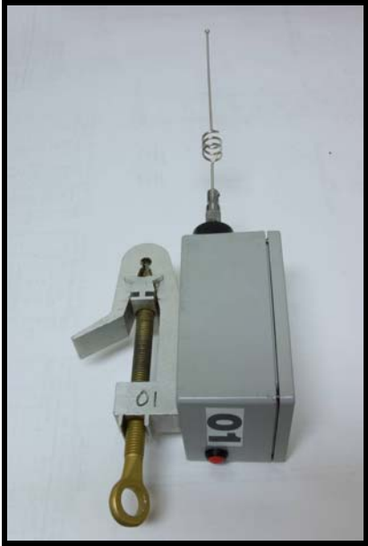
Figure 18. Redesigned BSI with metallic antenna and switch
