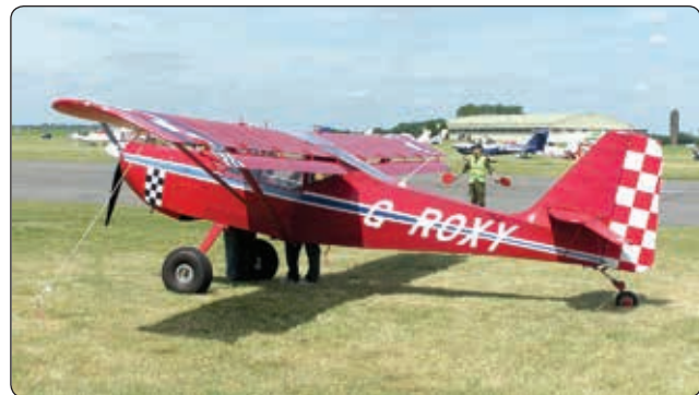
Figure 6-9. Flaperons on a Skystar Kitfox MK 7.
