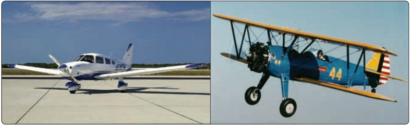
Figure 3-6. Monoplane (left) and biplane (right).
