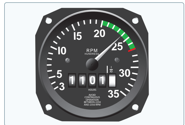
Figure 7-8. Engine rpm is indicated on the tachometer.
