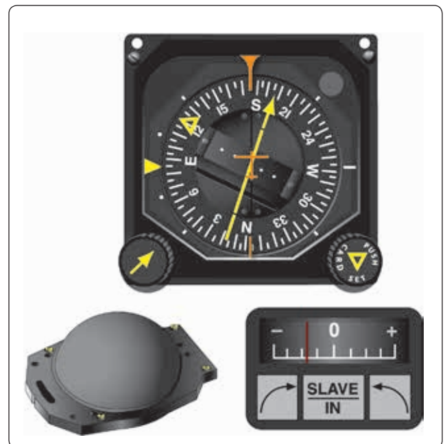
Figure 8-29. Pictorial navigation indicator (HSI, top), slaving meter (lower right), and slaving control compensator unit (lower left).
