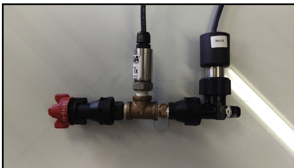
Fig. 2 – Nozzle body and pressure transducer assembly used to measure nozzle tip pressures after the pulse-width modulation solenoid valve. Another pressure transducer was connected inline 40-cm upstream from this assembly to provide gauge application pressure.
