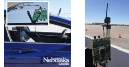
(a) Tx USRP on the roof-top (b) Rx USRP behind the barrier
