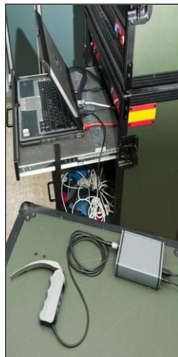
Figure 5. The Karl Storz C-HUB and C-MAC Videolaryngoscope connecting by USB to the telemedicine computer.
