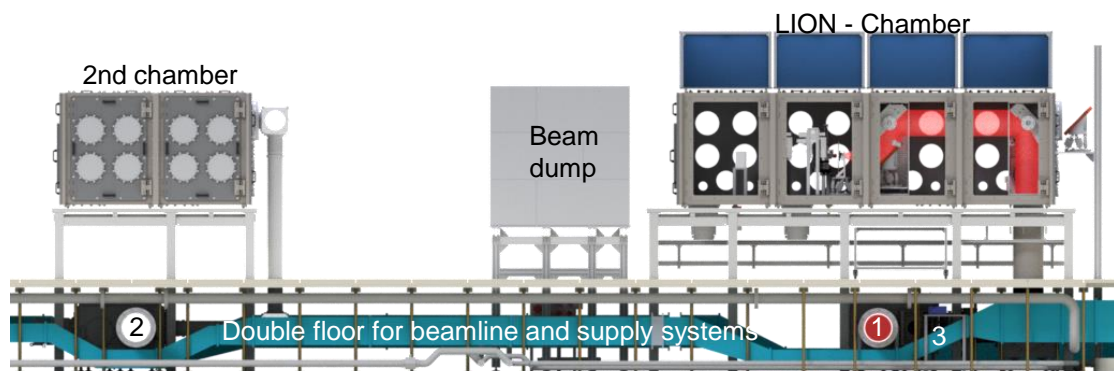
Figure A.16 | The LION cave. The double floor is hosting the LBD and supply cables for water, air conditioning, gases, electricity and signal cables. The laser (1) enters the cave in the double floor and is then guided to the vacuum chamber. A second arm of the beam line (2) can be used to guide, for example, the ATLAS-300 laser into the 2nd chamber that can be used for smaller experiments and test purposes. A CW diode laser of 1 W with 3 cm beam diameter can be coupled in for alignment purposes (3). The beam dump strengthens radiation safety outside the cave during full operation of LION.
