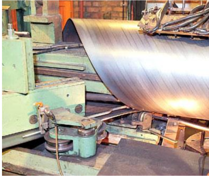
Figure 1.9: Helix forming of spiral welded pipe [Hall Longmore]
