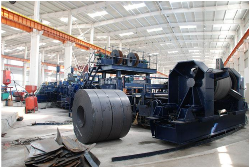
Figure 1.8: Carbon steel coil used for spiral welded pipe production
