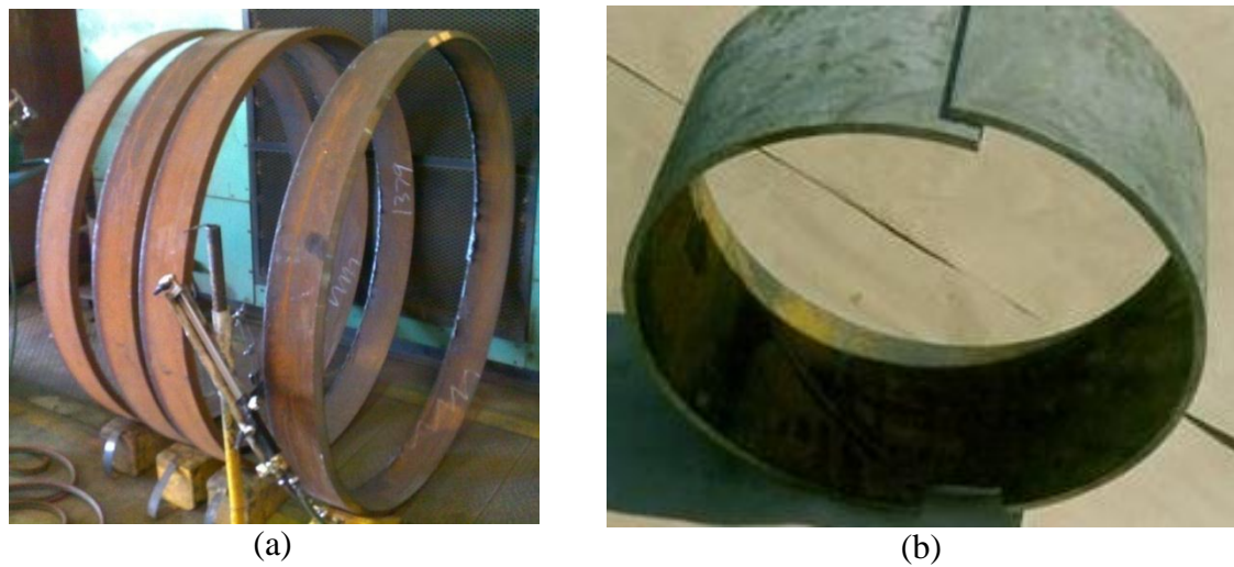
Figure 3.2: (a) Preparation for splitting ring test, (b) Ring cut from spiral welded pipe.
