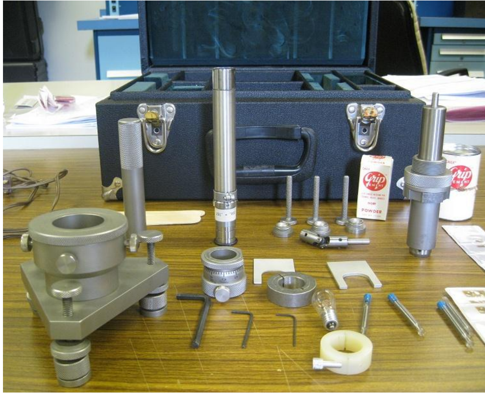
Figure 1.32: RS-200 mill guide used for drilling hole technique
