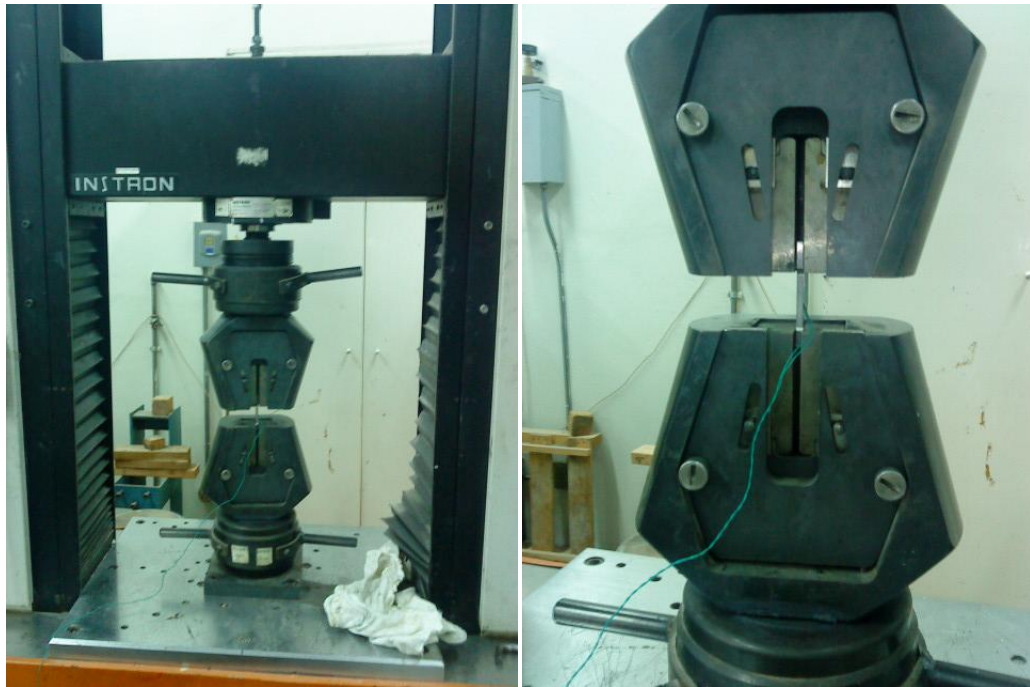
Figure 3.4. Mounting the specimen on the tensile testing machine
