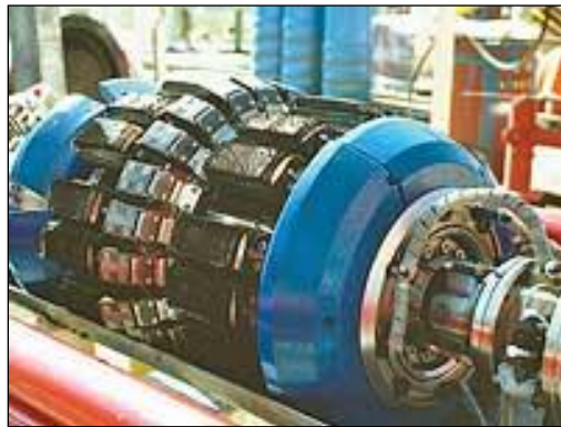
Figure 1.8. Picture of MFL tool (ROSEN 2007, CDP)
