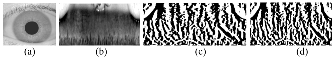
Figure 9: Iris sample image (a), Normalized iris image (b), Real part of Gabor-based iris decomposition (c), Imaginary part of Gabor-based iris decomposition (d)
