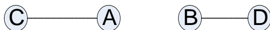
Figure 2-1: S-MAC: Neighboring nodes A and B have different schedules. They synchronize with nodes C and D respectively
