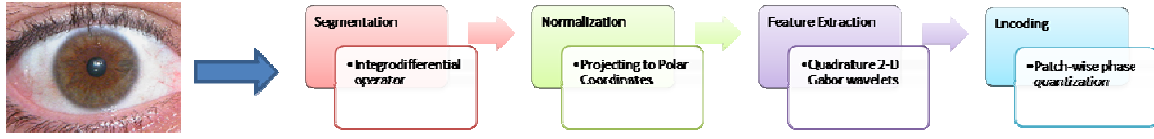
Figure 2.2: Process of Daugman algorithm.
