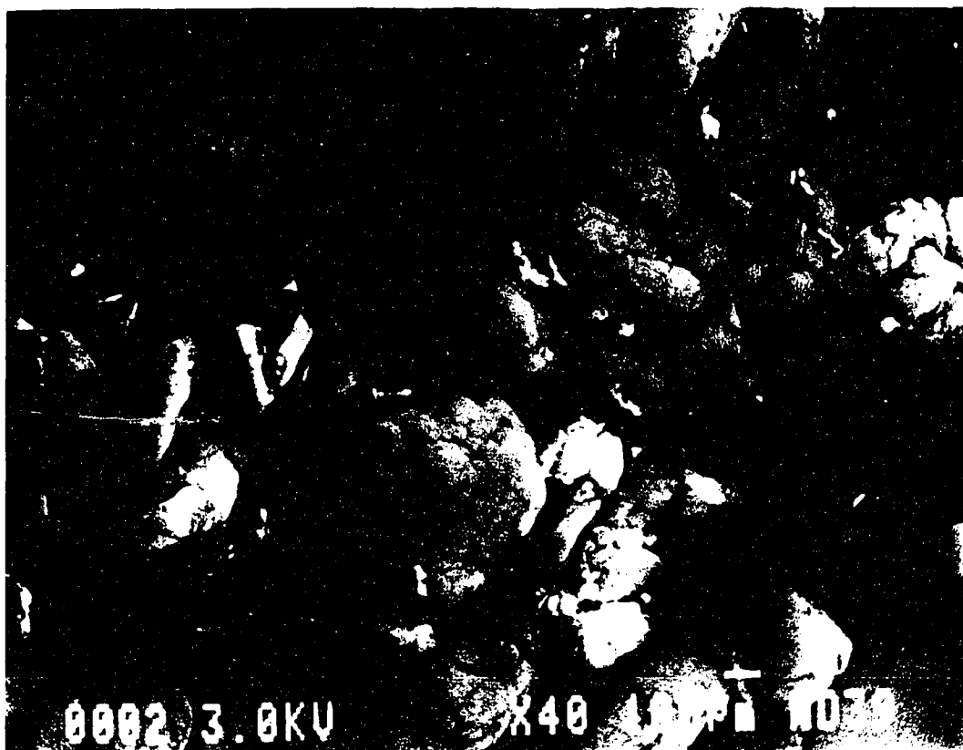
Fig. 4.2 : SEM Micrograph of PTFE Particles
