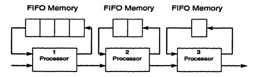
Figure 2.10: Radix 2 eight-point FFT with decimation in time.
