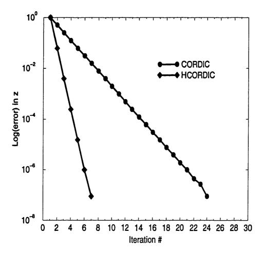
Figure 5.4: Comparison between the standard and the new CORDIC in the convergence rate of z in the vectoring operation of the linear mode, where (x, y, z) = (3, 1, 0).
