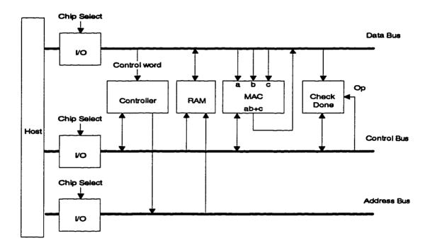
Figure 6.3: Architecture of the HCORDIC processor.
