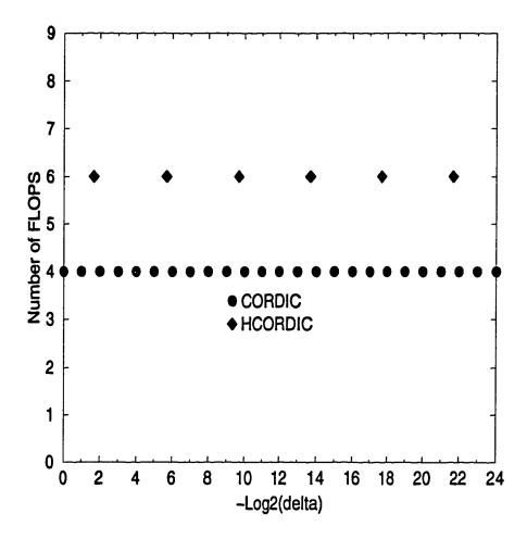
Figure 5.5: Plot of the number of operations at each CORDIC iteration, where the operation is vectoring in the linear mode, and (x, y, z) = (3, 1, 0).
