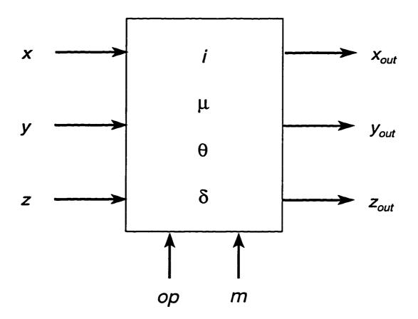
Figure 2.1: Block diagram description of CORDIC.
