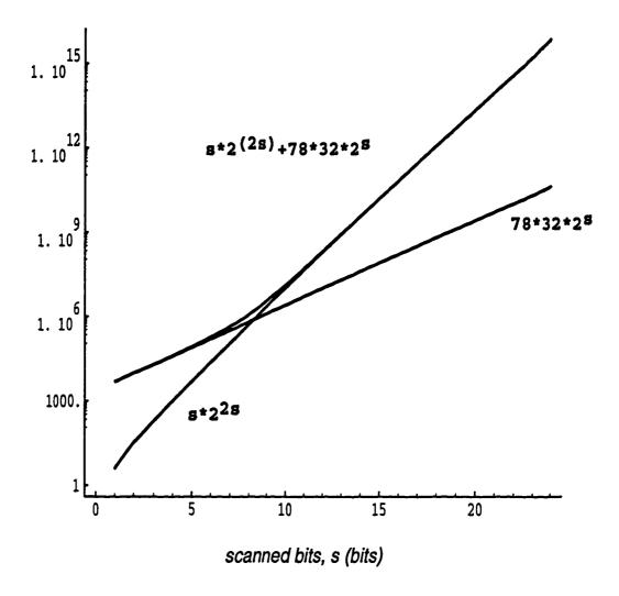
Figure 4.1: Effect of the number of bits scanned in parallel, s, on the look-up table size .
