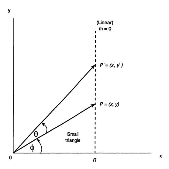
Figure 2.3: Rotating a vector by  $\theta$  in the linear mode, where  $\phi$  is the initial "angle" and R is the "radius" of the vector P = (x, y).
