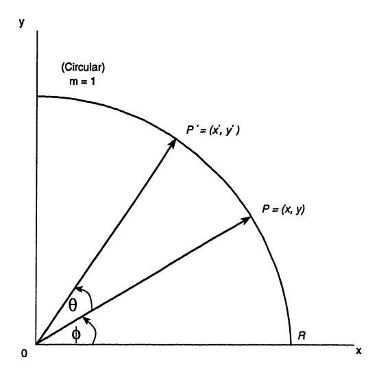
Figure 2.2: Rotating a vector by  $\theta$  in the circular mode, where  $\phi$  is the initial angle and R is the radius of the vector P = (x, y).
