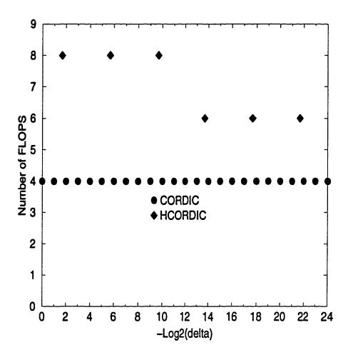
Figure 5.3: Plot of the number of operations at each CORDIC iteration, where the operation is rotation in the circular mode, and  $(x, y, z) = (2, 0, 30^{\circ})$ .
