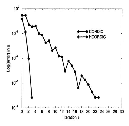
Figure 5.2: Comparison between the standard and the new CORDIC in the convergence rate of x in the rotation operation of the circular mode, where  $(x, y, z) = (2, 0, 30^{\circ})$ .
