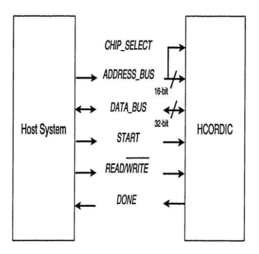
Figure 6.1: Interface between the host system and the HCORDIC processor.
