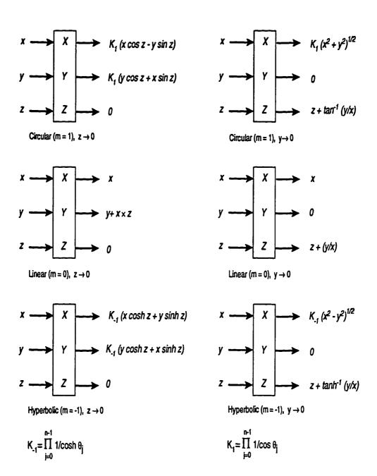
Figure 2.5: Input-output block diagram of CORDIC.
