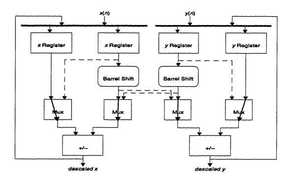
Figure 2.7: CORDIC descaling unit.
