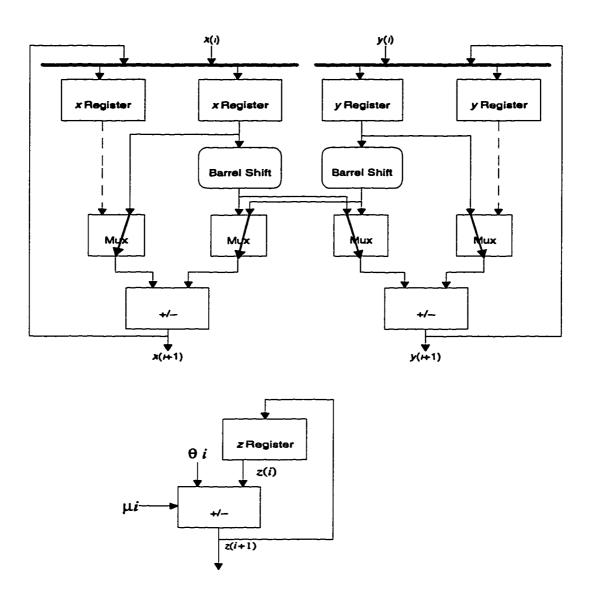
Figure 2.6: Basic CORDIC processor.
