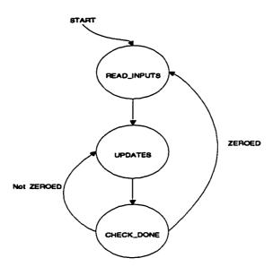
Figure 6.5: State diagram of the HCORDIC controller.
