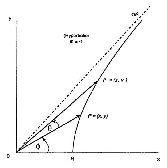
Figure 2.4: Rotating a vector by  $\theta$  in the hyperbolic mode, where  $\phi$  is the initial "angle" and R is the "radius" of the vector P = (x, y).
