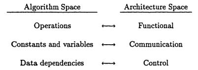
Figure 6.2: Mapping of the design issues in the algorithm space and the corresponding architecture space.
