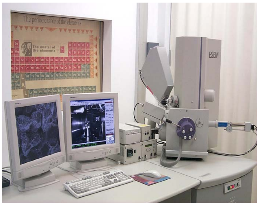
Figure 3.6 Photograph of ESEM (Philips XL-30).
