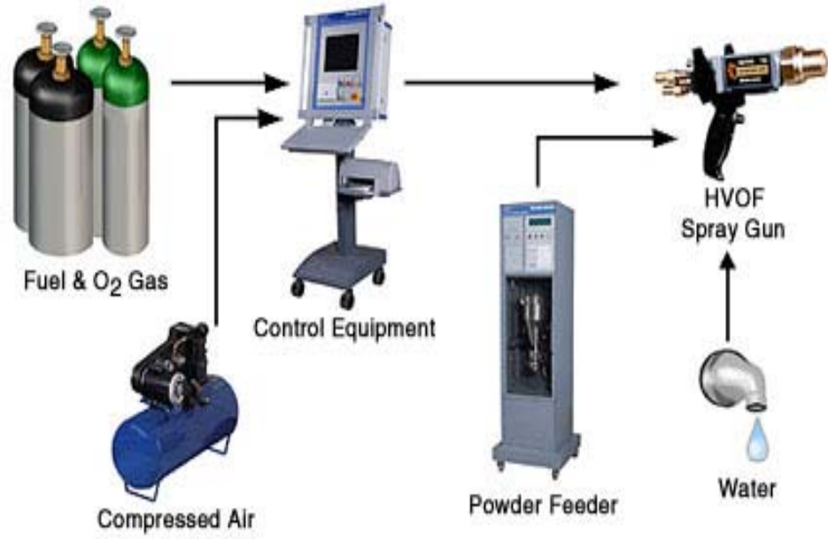
Figure 3.1(a) High velocity oxygen fuel system (Sulzermetco, 2002).
