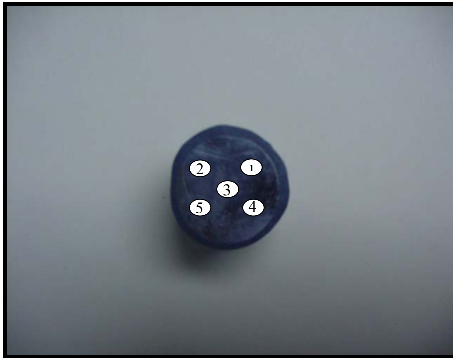
Figure 4.21 Photograph showing the 5 points where microhardness is measured at the sample coating surface.
