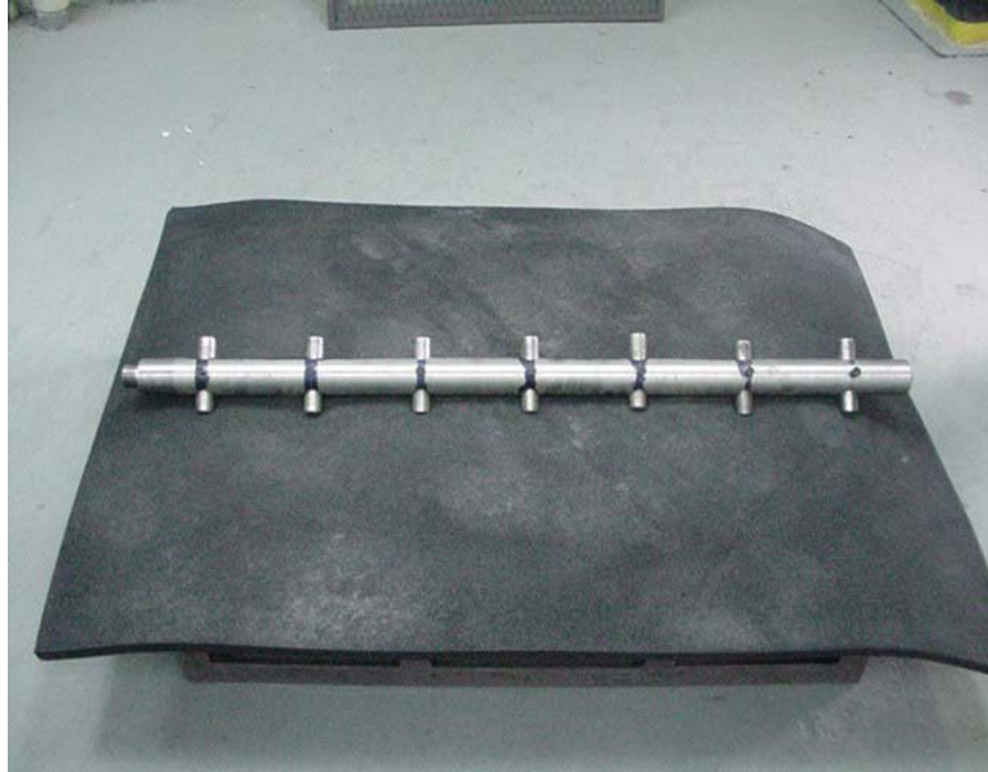
Figure 3.11 Preparation setup of the sample for tensile bond strength.
