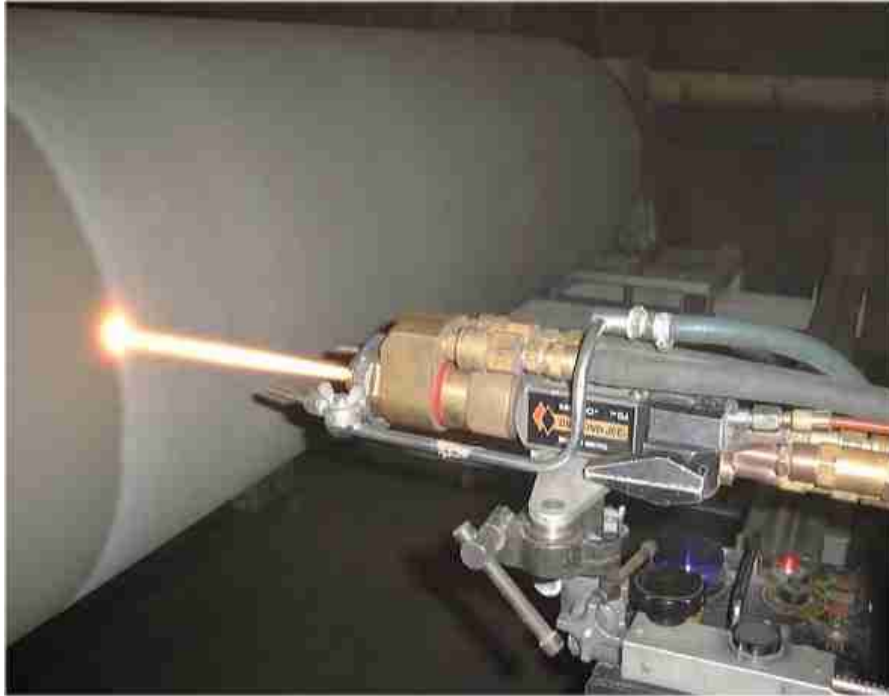
Figure 3.2 Photograph of the HVOF system and the work piece during spraying.
