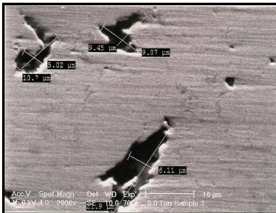
Figure 4.9 SEM image showing the porosity sizes for coating 3 at 2000x.
