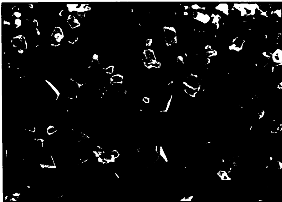
Figure (4.8): Surface morphology of Incoloy 803 after 100 hours of exposure in air at 800°C.
