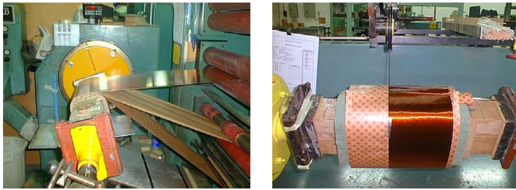
Figure 3.7 LV winding (left side) and HV winding (right side) during manufacturing
