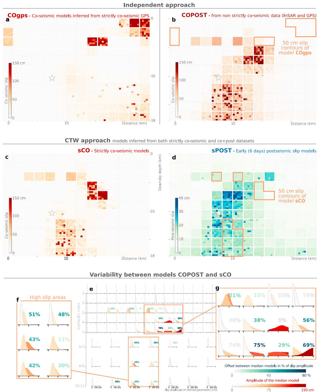
Figure 3. Comparison between finite-fault models inferred with the independent or the CTW approach. (a) Strictly coseismic (30 s after the mainshock) slip model, named COgps, inferred from the strictly coseismic data set (GPS only). (b) Nonstrictly coseismic model COPOST inferred from the coseismic data set contaminated with some postseismic deformation. (c and d) Strictly coseismic sCO and early postseismic sPOST (6 days after the mainshock) slip models inferred jointly with the CTW approach. (a) to (d) illustrate the slip amplitude of the median models (norm of the slip vector) of 25 families of inferred models (more information in the text and Figure S3). Each subfault (large square) is divided into 25 pixels colored from the slip amplitude of the corresponding median model. (e) Comparison between the posterior probability density functions of the dip-slip parameters of models COPOST (b) and sCO (c), colored from the amplitude of their median model. In the last four rows, the PDFs have been merged, covering two subfaults along strike and two subfaults along dip (i.e., patches 2 times bigger than for the first four rows). The COPOST model PDFs are in the background, while the sCO PDFs are in the foreground. The offset between the median models is shown as percentage with a different color scale. Two high slip areas are illustrated in detail: the highest slip patch (g) and the deep slip patch (f). The plots of the posterior PDFs are truncated between 0 and 200 cm to simplify the visualization. CTW = Combined Time Windows.
