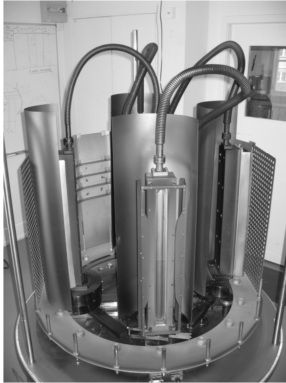
Fig. 1. The coating facility at DNSC with four cathodes. The cathode in the front and to the right is in the “open” position, ready to sputter where the one to the left and the one in the back are in “close” position. The samples are mounted on mounting plates placed on the big ring in the bottom, the front half of the mounting plates have been removed. There are 16 mounting plates and two dummy plates on the ring. The targets in the cathodes are 500 mm tall, 38 mm wide, and the ring is a little over one meter in diameter.
