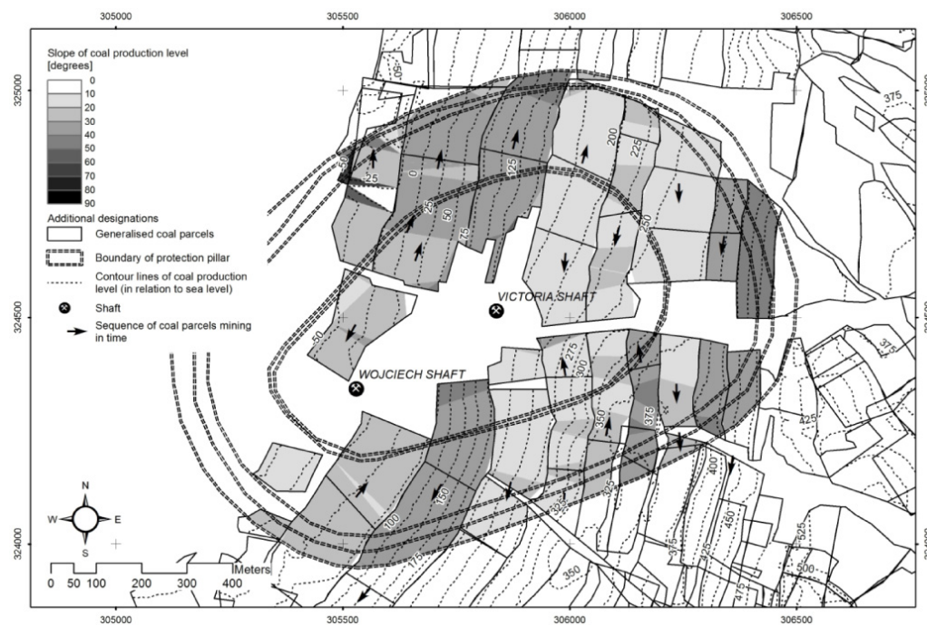
Figure 11. Slope analysis for the 424/425 coal production level within the boundaries of the protection pillar.
