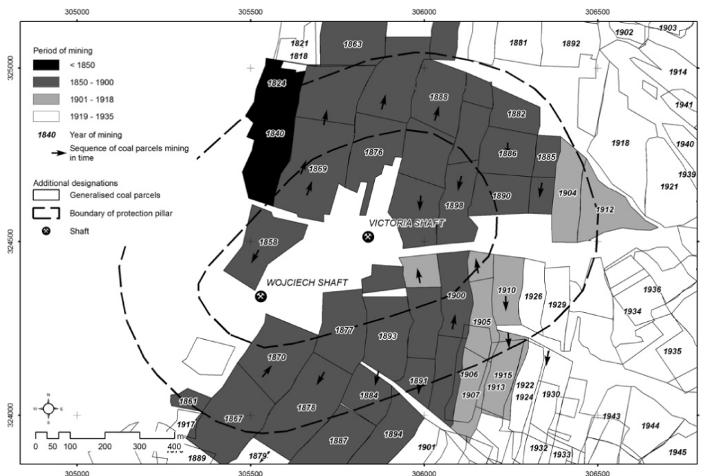
Figure 10. Mining activity analysis for the 424/425 coal production level within the boundaries of the protection pillar.
