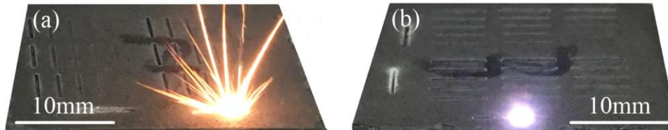
Fig. 13. Ablation process of femtosecond laser on the SiC/SiC surface: (a) photothermal effect, (b) photochemical effect.
