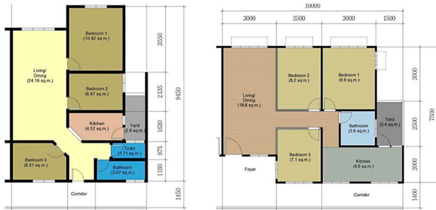
Figure 4. The unit plan layouts for the People’s Housing Programme (PPR) first-generation units (left) and the new proposal for the ‘airhouse’ standard (right) [4].
