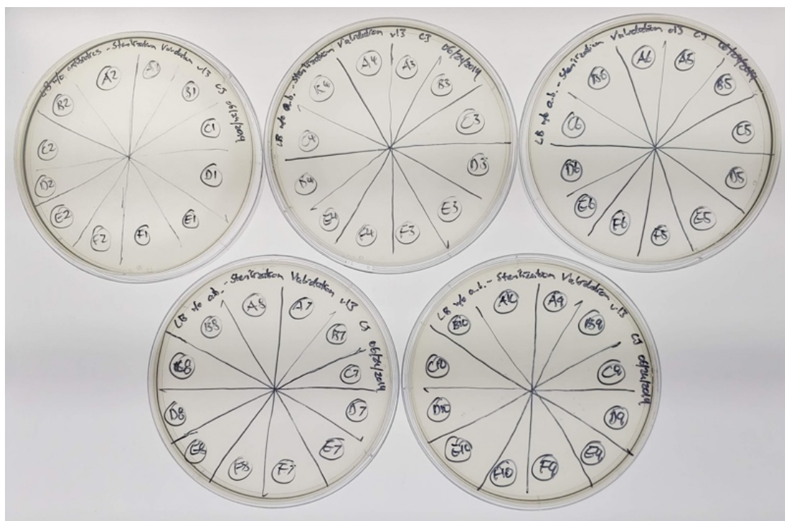
Figure 10: Sterilization validation v13 demonstrates no contamination in any of the wells proceeding 72hr culture and sterilization.
