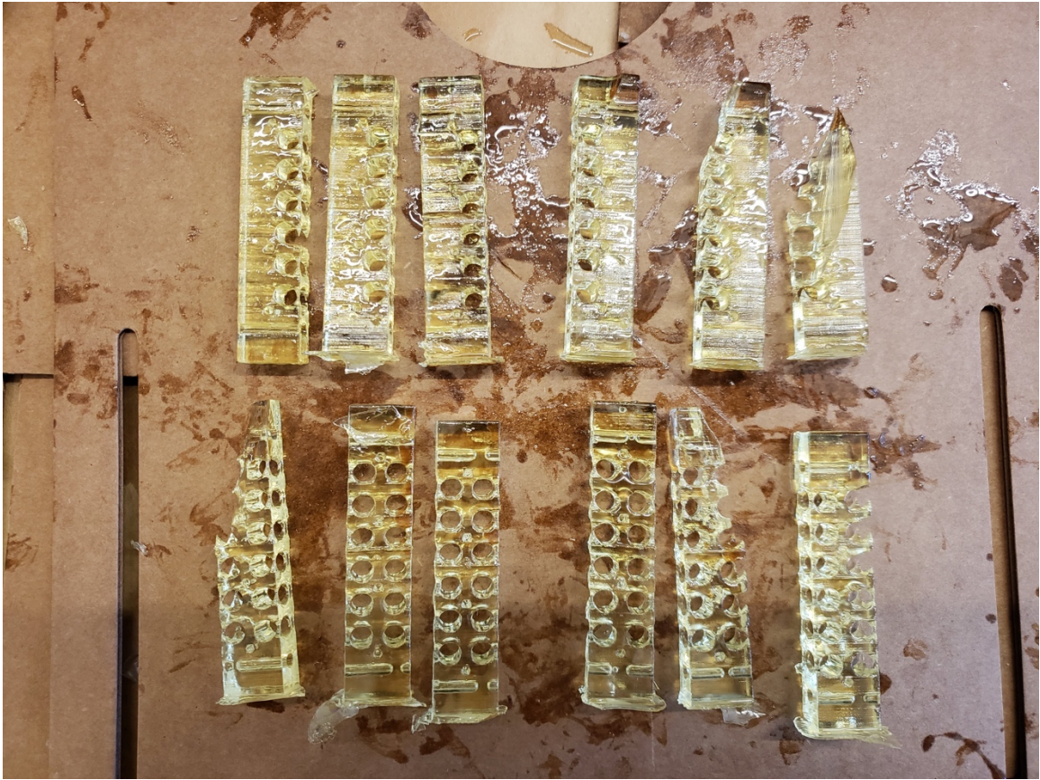
Figure A4: Example of failed body segment prints using the Form2 printer and Formlab's Dental SG Resin
