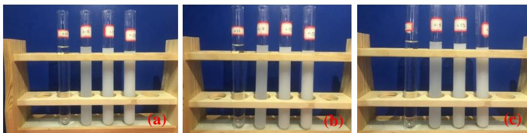
257 Fig. 2. \text{SiO}_2\text{-water} nanofluids at different quiescent time, (a) just prepared, (b) 258 laying up 10 days, (c) laying up 20 days
