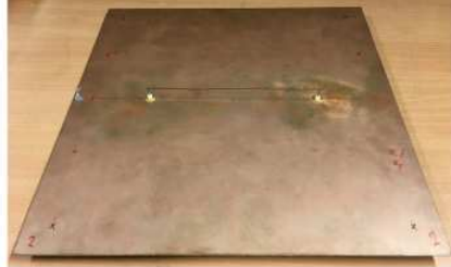
Fig. 3. A DUT consists of double loop structure to calibrate probes. (a) With probe RF-R50-1. (b) With probe RF-R0,3-3.
