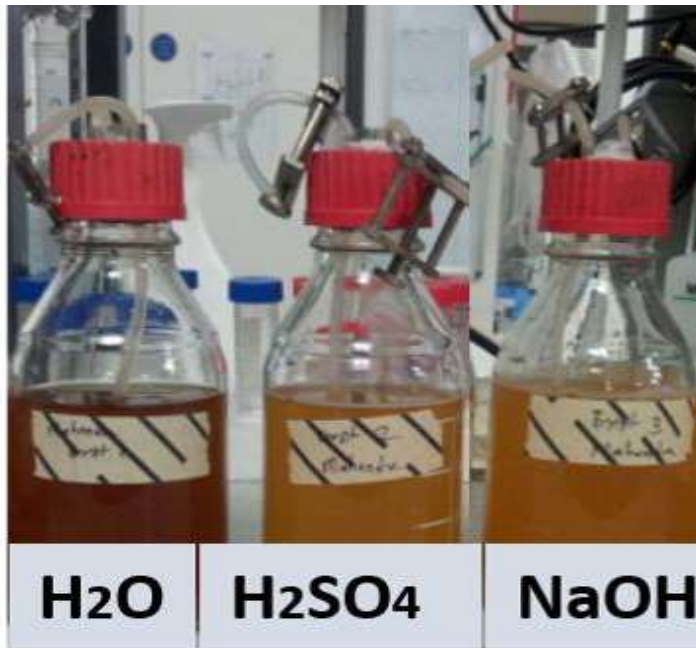
Fig. S2 Experimental set-up of the fermentation of miscanthus biomass hydrolysate using C. acetobutylicum .
