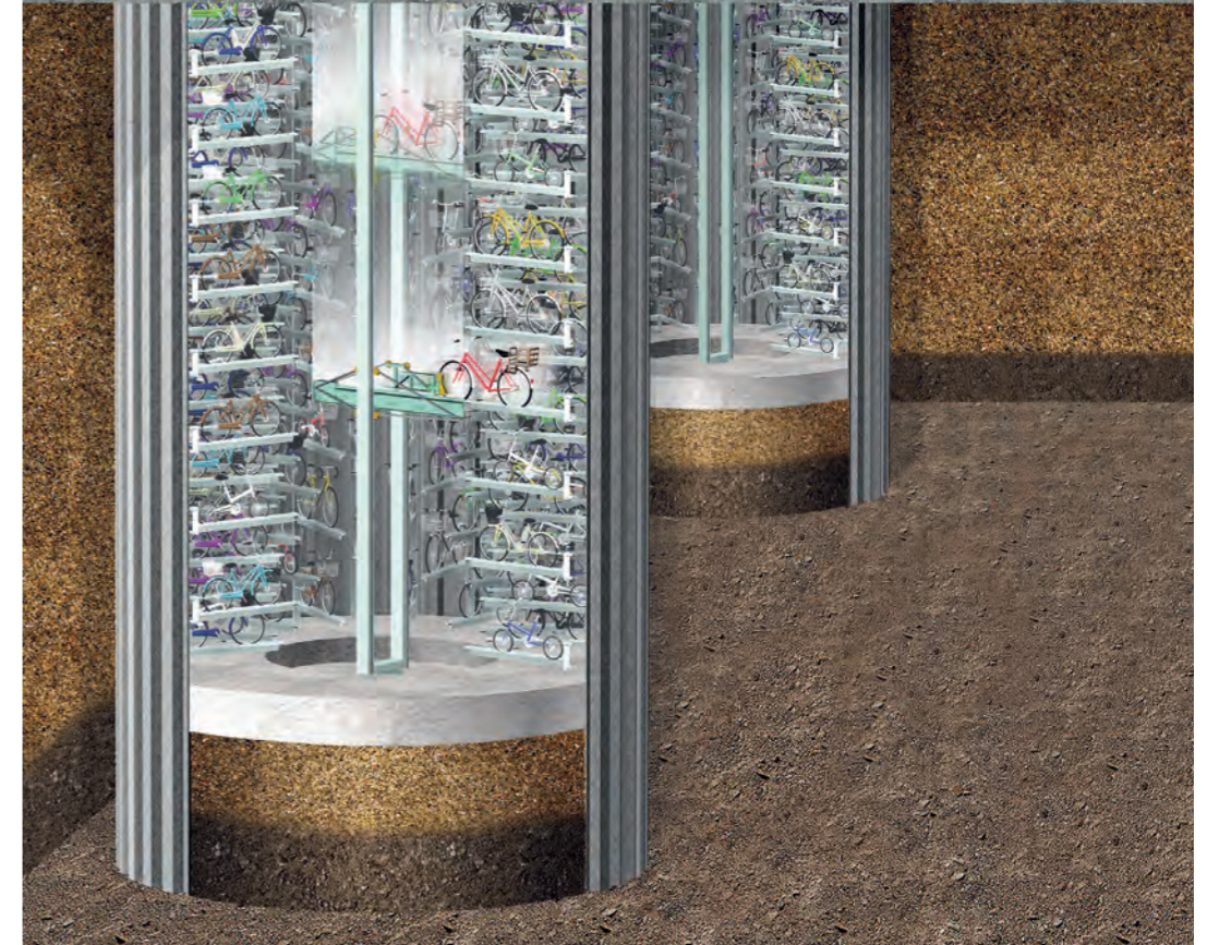
Giken underground eco-cycle parking system, Tokyo
