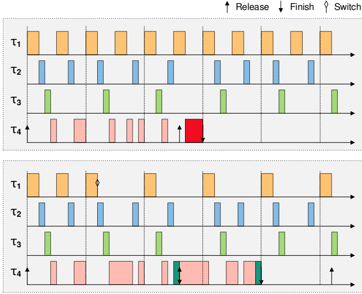
Fig. 5. Converting \tau_1 into a dual-mode task makes an unschedulable task set (the top diagram, note the red block) schedulable (the bottom diagram). All tasks are released at the same time.
