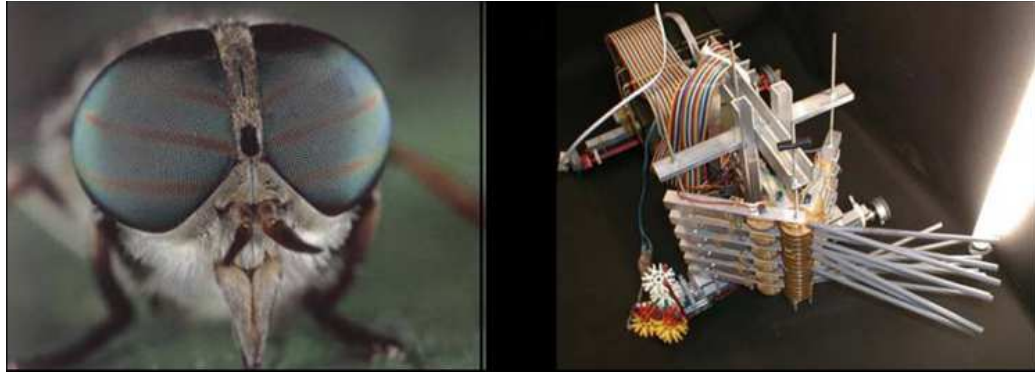
Figure 8. Eyebot (right), a reconfigurable robot inspired by the insect compound eye (left), designed to apply artificial evolution to robot morphology. Figure from (Pfeifer & Gómez, 2009).
