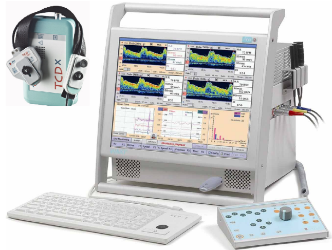
FIGURE 1 – Portable TransCranial Doppler (TCD) system and a TCD holter from Atys Medical.
