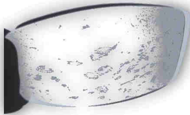
Delamination after Process Modification
