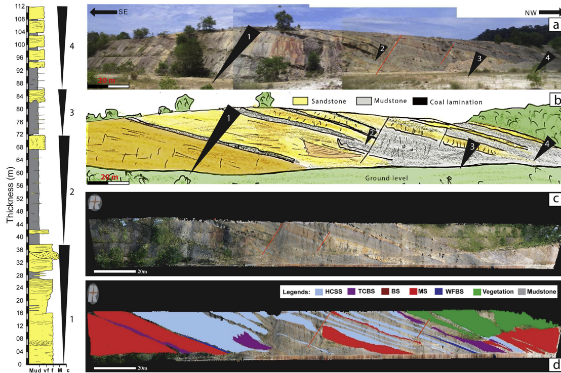
Figure 6. The hierarchy of four coarsening upward units (stratigraphic log at left) with outcrops; (a) and (b) outcrop photograph and sketch representing the units and lithology (sandstone, mudstone and some coal lamination) distribution with two normal faults marked between units 2 and 3; (c) LiDAR point cloud with texturing of high resolution photograph represent the full section, the mudstones show thickness of <1 m thick and sandy facies, which thicken upward, vary from 10 m thick at base and thin up to 4 m towards the top of the unit; (d) detailed description of each of the sandstone facies static connectivity with different colors representing the thicknesses with its lateral and vertical extents.
