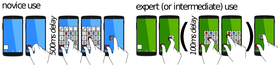
Figure 1: FastTapAdjust. In novice mode, users press the menu button and wait for the grid to appear, then select a command by tapping on a grid cell while holding the menu button. In expert mode, users tap the menu button and the command’s location with a two-finger chord. Intermediate mode uses the same chord-based invocation, but users can pause and display items around their selection, allowing them to adjust the chord before selecting.
