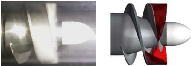
Figure 13. M1 Suction performance ( \sigma_c \approx 0.04 )
