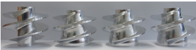
Figure 2. Inducers - from left to right: Ao, Mo, M1, M2
