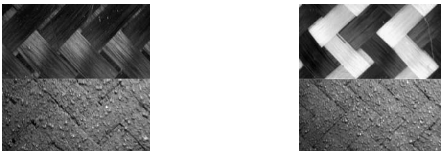
Fig. 1. Microscopic images before and after full treatment of Carbon Fiber Fabric (left) and Mixed Fabric (right)
