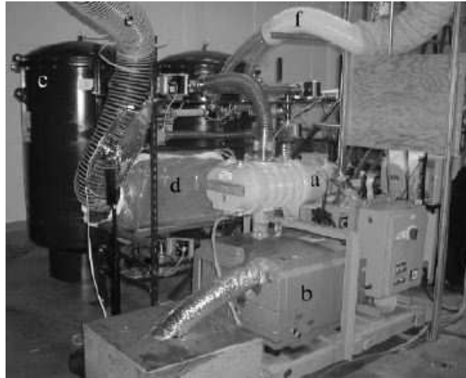
FIGURE 6. The radon filtered that supplied the entire make up air flow to the vessel assembly clean room. The device operated continuously for the whole year of vessel fabrication. The main components are labelled: a,b) vacuum pump (roots blower + backing pump, respectively), c) charcoal columns, d) hepa filter at the output, mounted in a frame together with the valve manifold, e) duct to the clean room, f) column repressurization line.
