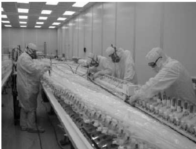
FIGURE 2. Gluing one of the joints of the IV. The large size of the clean room can be appreciated, as well as the effort made to cover all surfaces of the vessel not being bonded and to individually bag the clamps (used to apply pressure to the bonded panels during glue curing) to prevent particulate contamination of the vessel.
