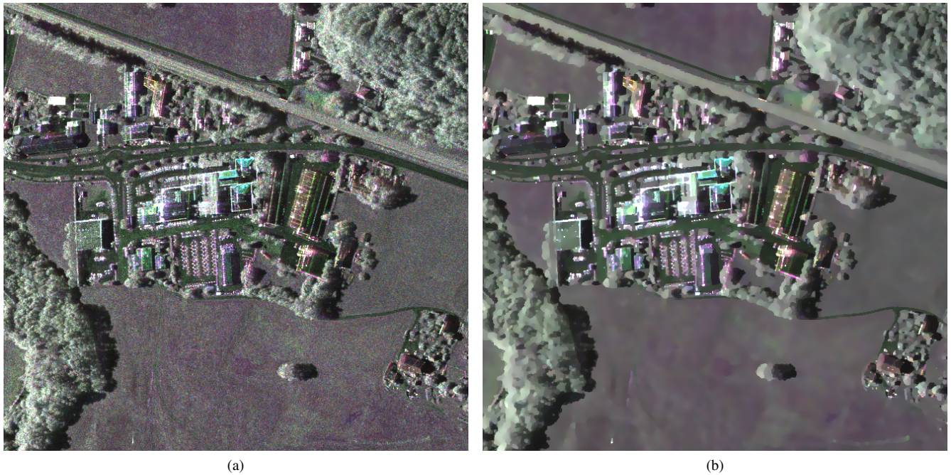
Fig. 12. Filtered polarimetric results from the X-band F-SAR (DLR), obtained from the Kaufbeuren 15OP15AF campaign, displayed using Pauli RGB color coding.
