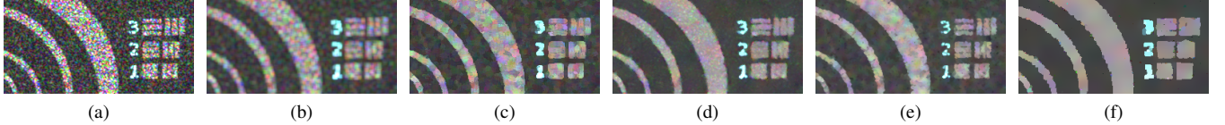
Fig. 6. Results over a cropped area comparing different speckle filtering techniques for the second synthetic case seen in Fig. 4(c). The spatially correlated SLC SAR imagery is presented in (a). In order to accommodate for the spatial correlation in the image, a 5 \times 5 boxcar filter was applied in (b). The filtering result of the refined Lee filter is showed in (c). Again, the results from the NL-SAR framework and IDAN filter in (d) and (e) respectively, show a moderate amount of smoothing of homogeneous areas and minimal loss of details. The result from our proposed method is showed in (f), where the filter achieves good edge reconstruction, however, the pre-processing step introduces artifacts that modify the small details and edges in the final result.
