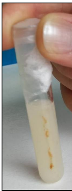
Figure 2.4. Sample MNP image. Representative image of freshly formulated PLGA/PVA coated \text{Fe}_3\text{O}_4 -MNPs.
