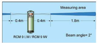
Figure 1. Illustration of the measuring area for the RCM 9 LW current meter
