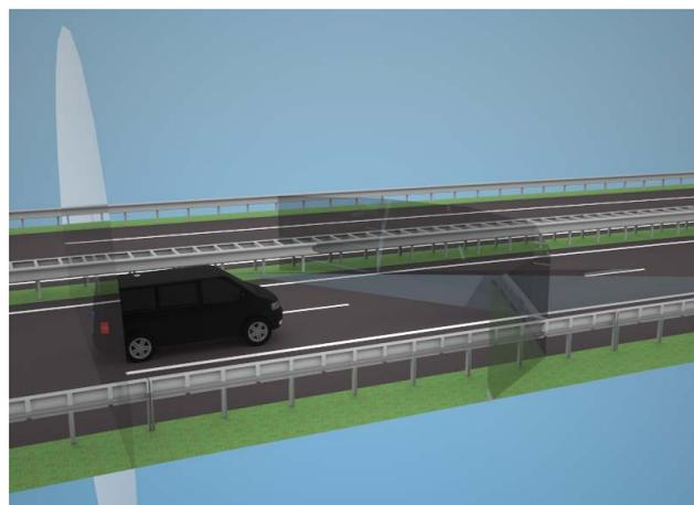
**Fig. 1.** The measurement vehicle is based on a Volkswagen Multivan witch was prepared to incorporate all sensors (5 cameras in front, lane mark detection system, high accurate positioning module with inertial measurement unit and a laserscanner).
