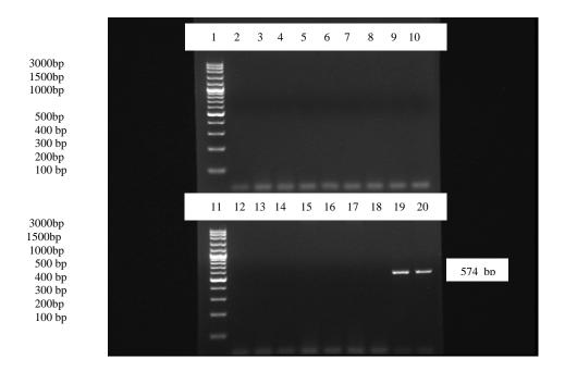
Fig. 2: PCR for the members of *M. mycoides* sub cluster showing an amplicon size of 574bp. Lane 1 & 11: Molecular Ladder; lane 2 -ve control; lanes 3, 4, 5, 6, 7, 8, 9, 10, 12, 13, 14, 15, 16, 17 and 18 test samples -ve for *M. mycoides* sub cluster members; lanes 19 & 20 *Mmm*LC and *Mmc* +ve controls, respectively.
