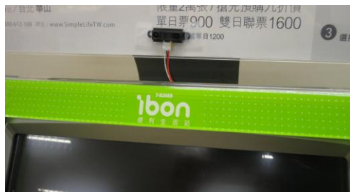
(a) An Infrared sensor on a iBon machine.
