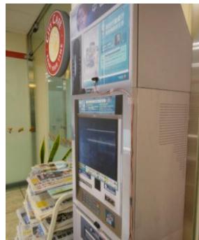
(c) An Infrared sensor on an ATM.
