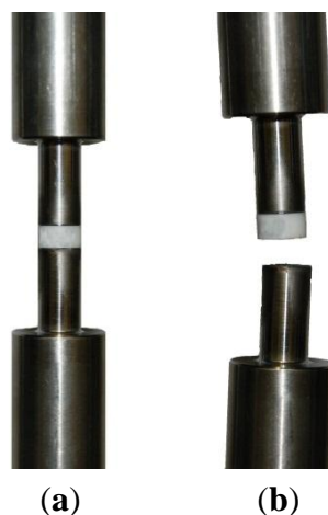
Figure 1. (a) Setup for adhesive strength test sample prior to testing; (b) Sample after testing.
