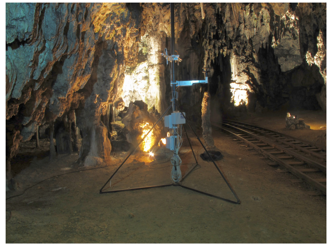
Fig. 5. Picture of static DTN node mounted by the railway in the cave where the train passes the cave meteorological station several times each day.
