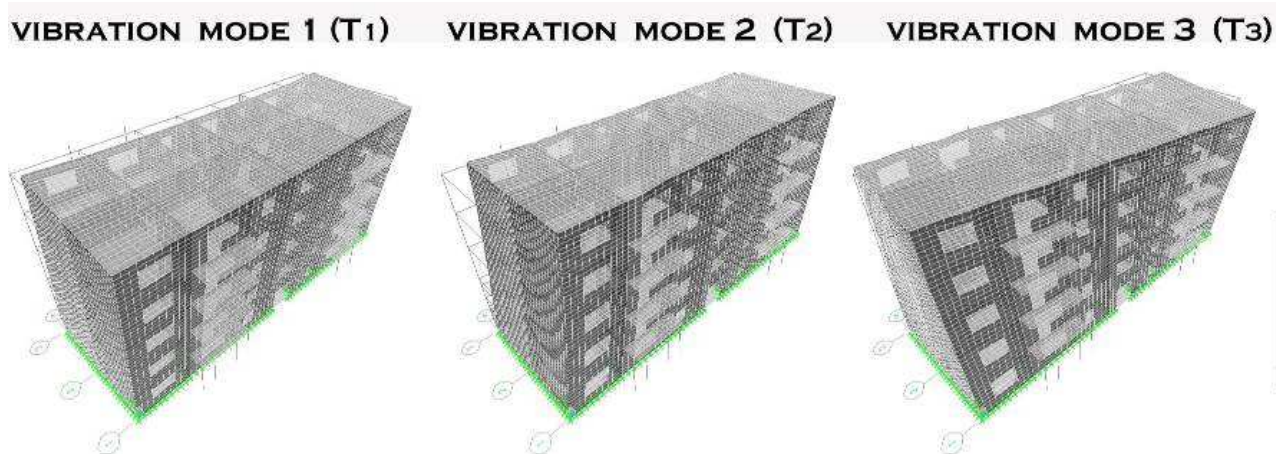
Fig. 5. Vibration modes and periods of original structure
