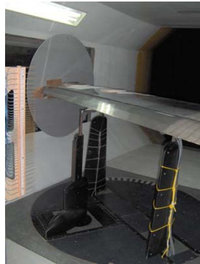
Fig. 11 Total heads rake with Gaussian distribution of probes, in the preliminary phase of WT campaign; large endplates
