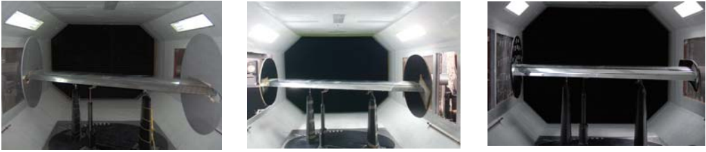
Fig. 12 SFWA 114 F15 model with large, intermediate and asymmetric (intermediate+small) end plates
