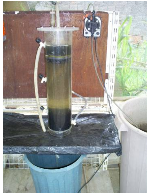
Fig. 2 (b) Picture of the Upflow Anaerobic Sludge Blanket (UASB).
